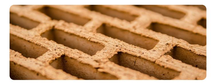
**Pollution absorbing bricks** suck in pollutants in the air and release filtered air. The innovative material is designed to be part of a building's standard ventilation system where the specialized brick is on the outside and regular insulation on the inside. These bricks have the potential to filter 30% fine particle pollutants and 100% coarse particles such as dust.
